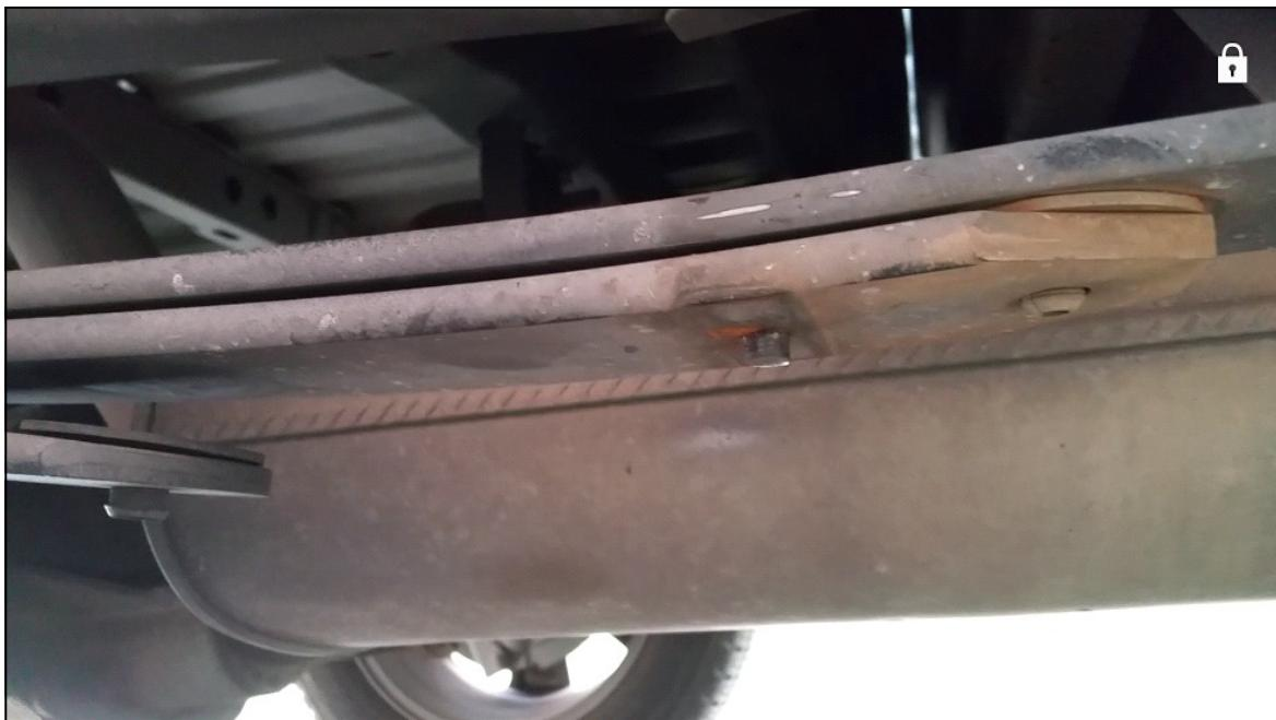
**Step 4.** Locate the forward bracket of your VAS Traction bar kit and install them on the leaf springs. Choose between the center hole and off set hole on the leaf spring mount and make sure that the bump stop located on the front of the forward bracket sits underneath the leaf spring bushing. See pic below for reference.
