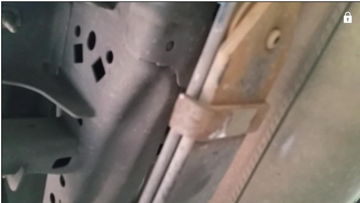
**Step 3.** Once the clamp has been removed it will expose a pin that is left over from the original rivet. This pin will be used to locate the forward bracket on the leaf spring.
