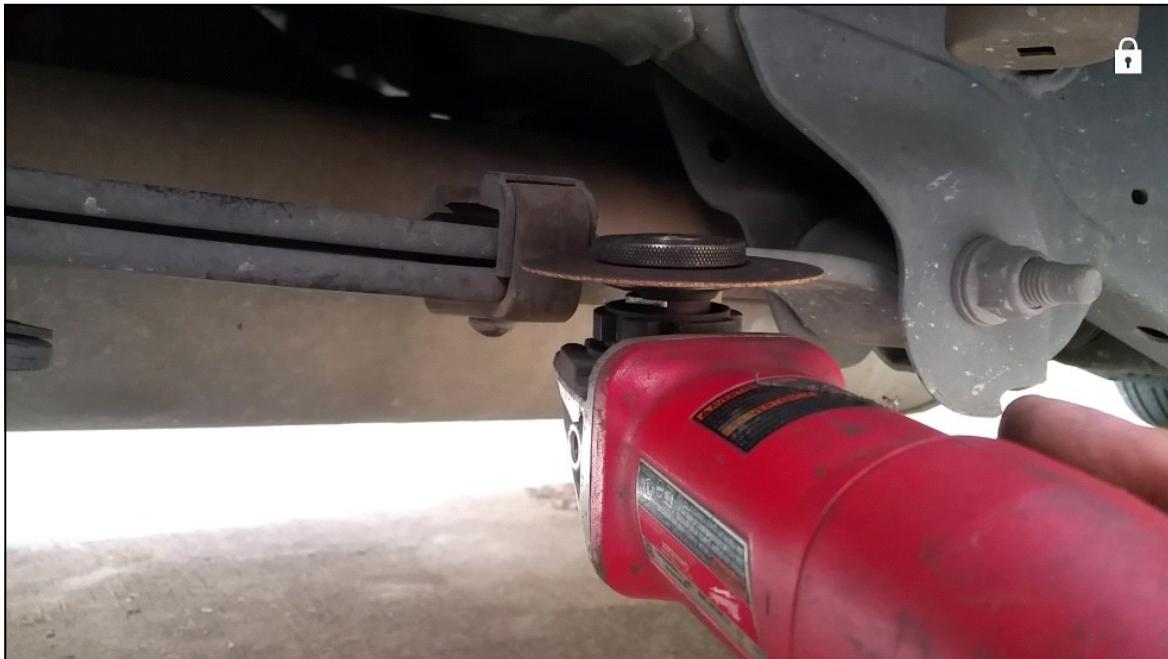
**Step 2.** Grind the rivet located at the bottom of the clamp. Once it is completely flush hit the clamp with a hammer and the clamp will fall right off. If you do not cut the top part of the bracket in step 1 you will need to pry open the clamp in order to remove it.
