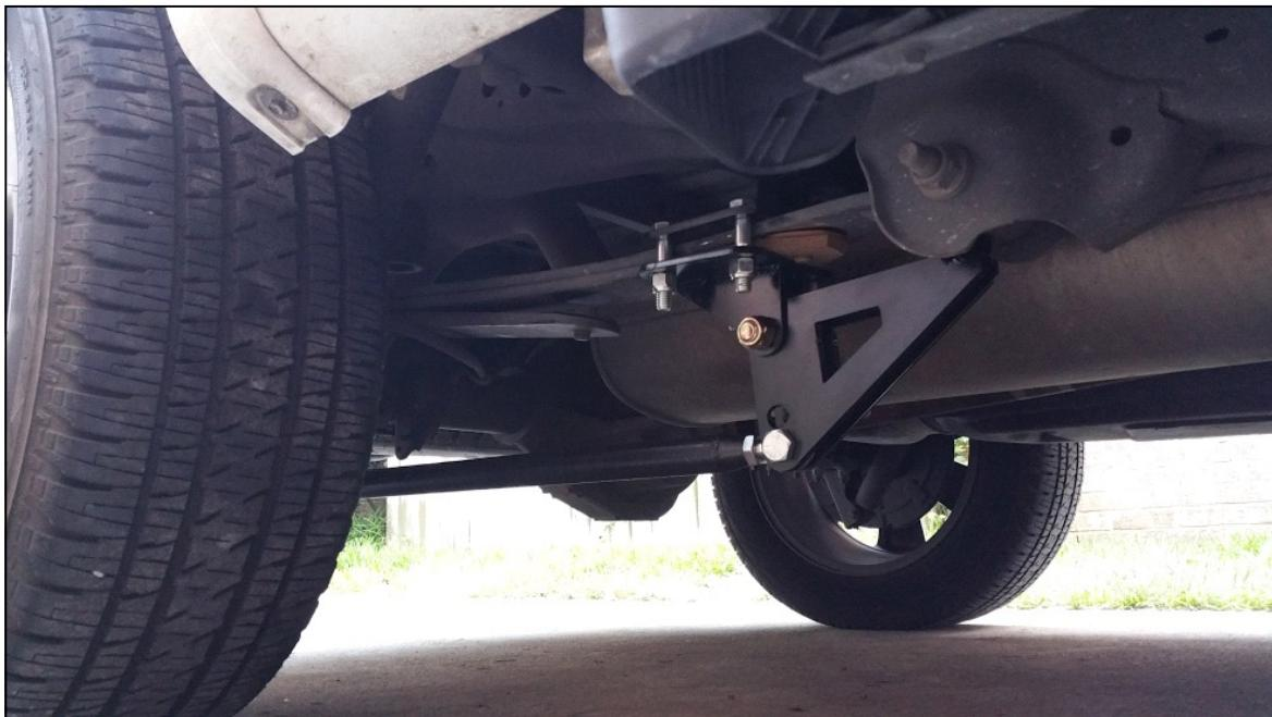
**Step 5.** Install the rear bracket as shown. Remove the 4 ubolt nuts and place the bracket underneath the stock axle bracket. Reinstall the nuts and tighten to specs. Ensure the flat part of the bracket is facing the front of the truck.
